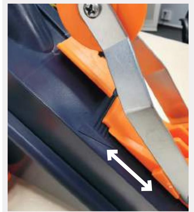
5/ Pull the tape until it is completely covered with compound.
