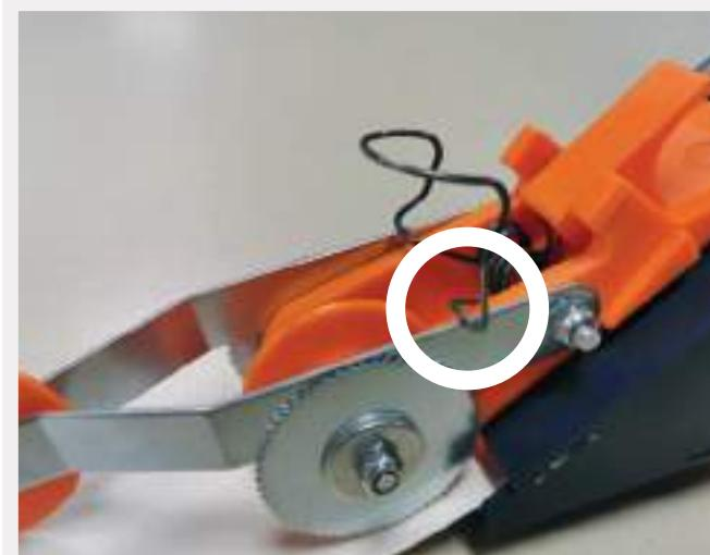
3/ Apply the tape, the roller will automatically fit into the angle.
