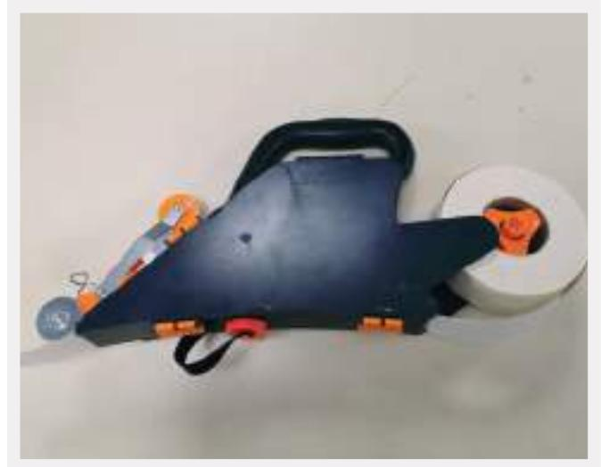
4/ Lift the lock a 1/4 turn to release the head.
