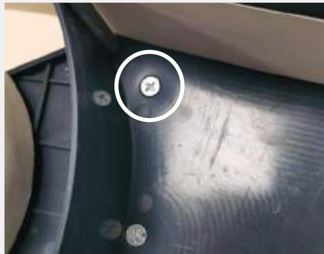
2/ Drill through the front holes using a Ø5.2 drill bit.
